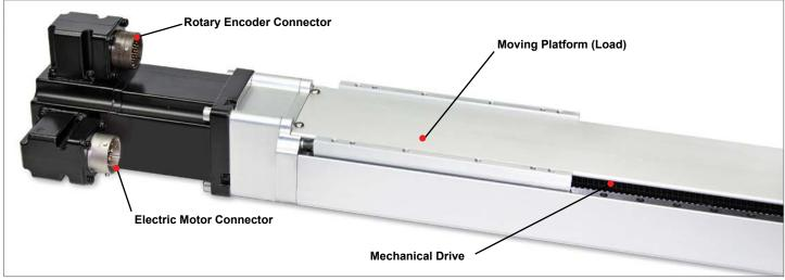
The indirect load monitoring system show in this application includes an electric motor directly coupled to a rotary shaft encoder, which acts as the load position sensor. In this setup, although the rotary encoder accurately indicates the drive motor's shaft position, the true standard of measurement is not the rotary encoder, but the drive system itself.
