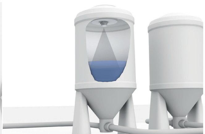
Level measurement of liquids in a tank using ultrasonic sensors
