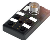
Passive distributors for collecting and consolidating the signals
